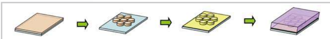
Figure 5 Schematic illustration of the fabricating process of P3HT/PMMA film coated on patterned Au/LSMO substrate: (a) coat LSMO resist on silicon; (b) create LSMO pattern by electron beam lithography; (c) evaporate Au thin film on the LSMO pattern; (d) coat P3HT/PMMA film on Au/LSMO pattern.
